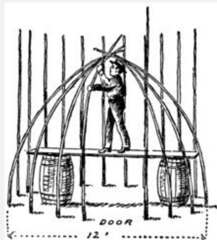
Fig. 131. Making the Frame of the Straw Hut.
