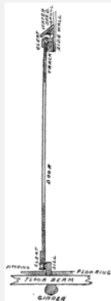
Fig. 144. Section of the Door and Frame.
