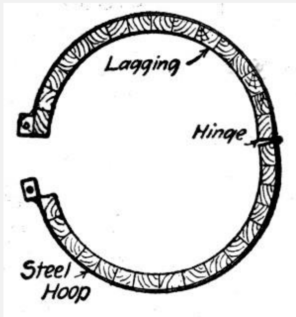
Fig. 189.—Form for Circular Column.
