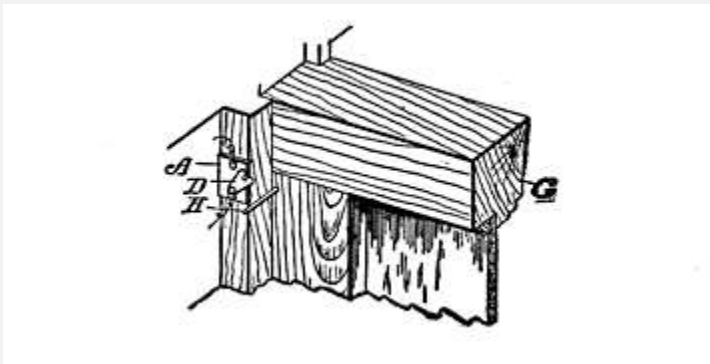
Fig. 55. ALARM SWITCH ON WINDOW
