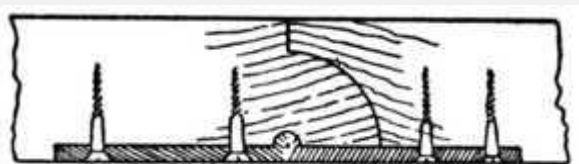
Fig. 250.—Rule Joint Hinge, with Leaf Open.
