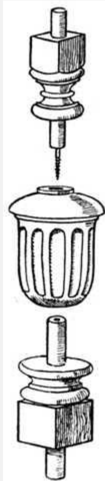
Fig. 349.— Method of Building up Turnings.
