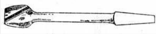
Fig. 196.—Dowel Rounder.
