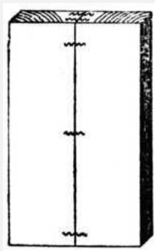
Fig. 362.—Jointing Boards.
