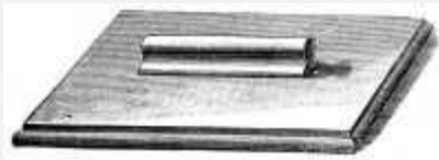
FIG. 239. FLAT PRESSER FOR LAYING ON THE PATTERN.
