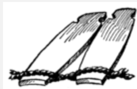
Fig 97. Barrel-stave Flooring.
