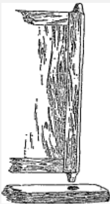
FIG. 76. Wooden pivot hinges of a Zuñi door.
